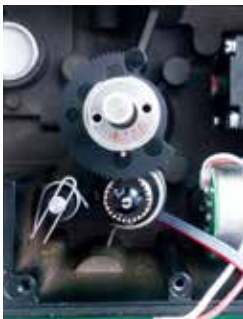
Potentiometer and cogwheel for 90° rotation
