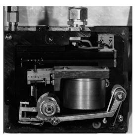
position of the spring (93) can be changed along the beam (92) and the balance arm (57) in order to adjust positioner gain, and thus the dynamics of the positioner. The positioner can be adjusted to match any small or large actuator.
