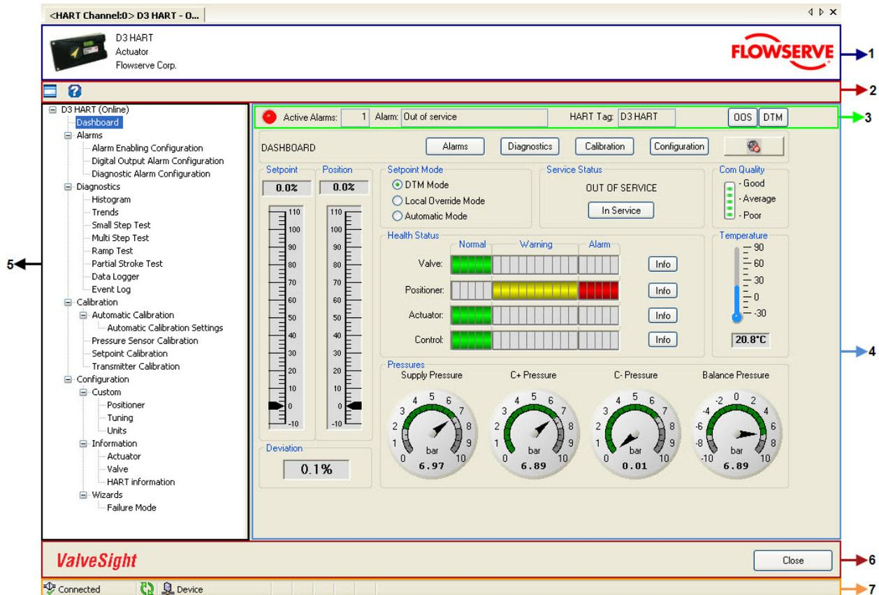
1. **Device Identification Area:** This area displays the picture of the D3 Positioner, type of device, and device manufacturer name.
