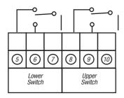
Connection of mechanical and proximity switches. (S,P)
