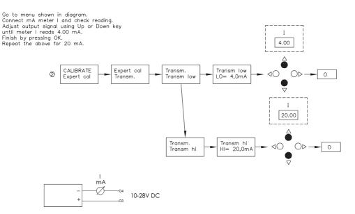
4-20 mA transmitter value will not be displayed in D30 LED. Only on external mA Meter.
