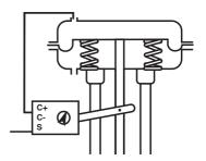
Double acting positioner, Direct function Double acting actuator
