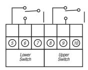
Connection of mechanical and proximity switches. (S,P)
