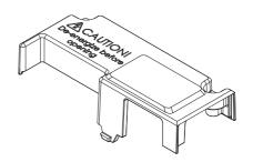
When installing the switch card, make sure it is placed correctly. Secure the PC Board with the two screws holding the plastic cover. Make sure the holes are centered before tightening the screws. Torque the screws to 0.3 Nm.
