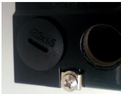
Use a coin to remove the black plug
