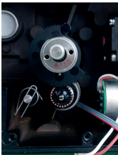
Potentiometer and cogwheel for 90° rotation
